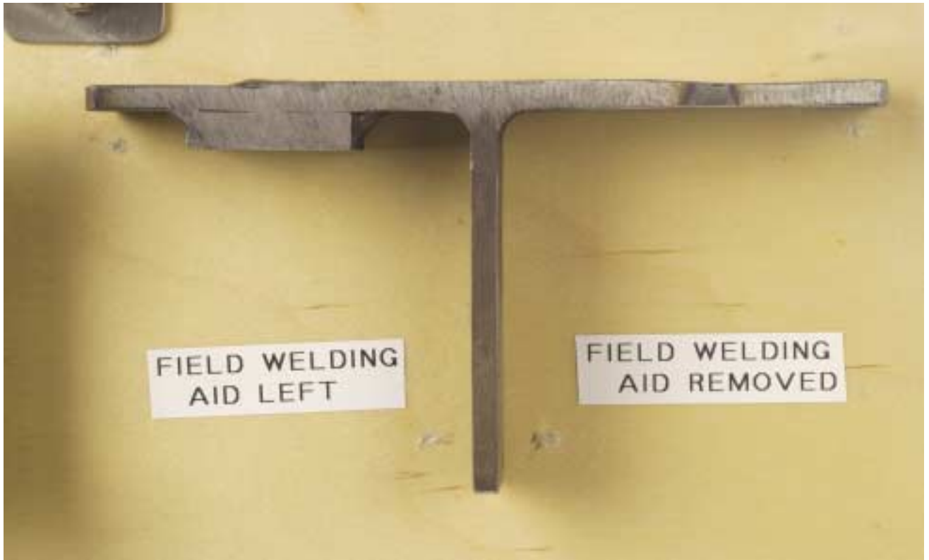
On the left, the field-welding aid (the backing bar) has been left in place. On the right, the field-welding aid has been removed and the weld ground smooth.
