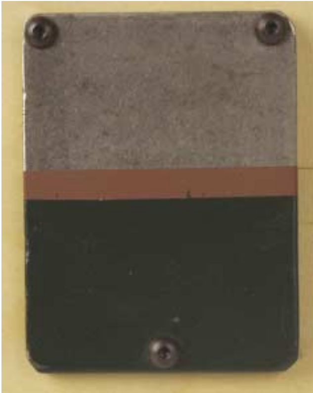
Low-end primer/finish coating: acrylic (water-based) finish coat with a shop coat primer over an SSPC-6 surface preparation.
