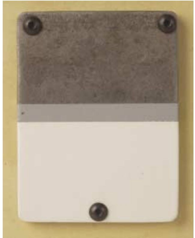
High-end primer/finish coating: epoxy finish coat with an epoxy or zinc rich primer, over an SSPC-3 surface preparation.
