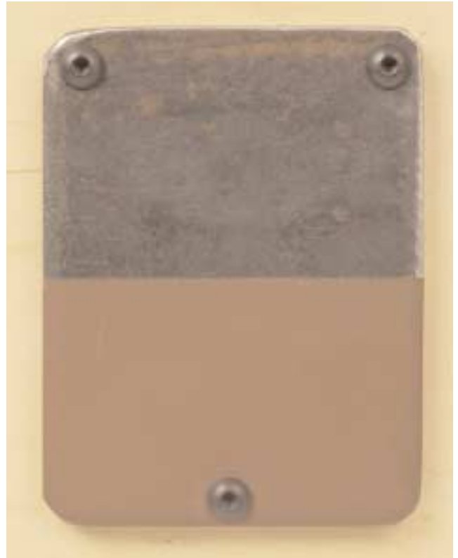
The appearance of sheared edges that have been ground.
