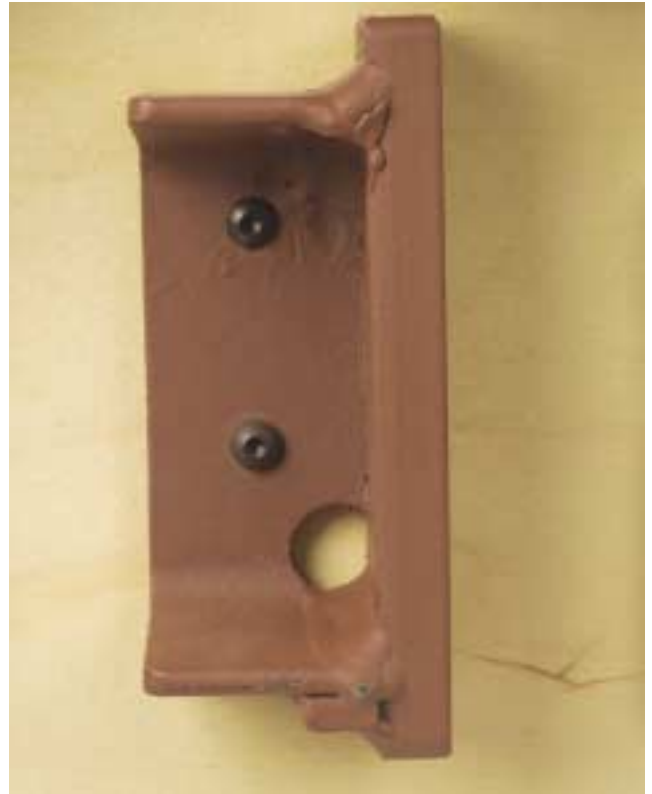
This sample shows a typical weld-access hole.
