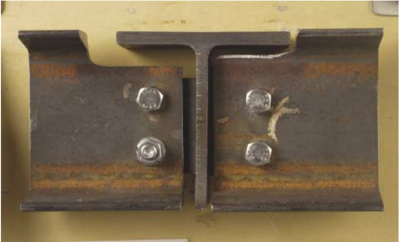
The connection on the left shows a connection with the typical blocking tolerance. The connection on the right shows the same connection with tolerances minimized.
