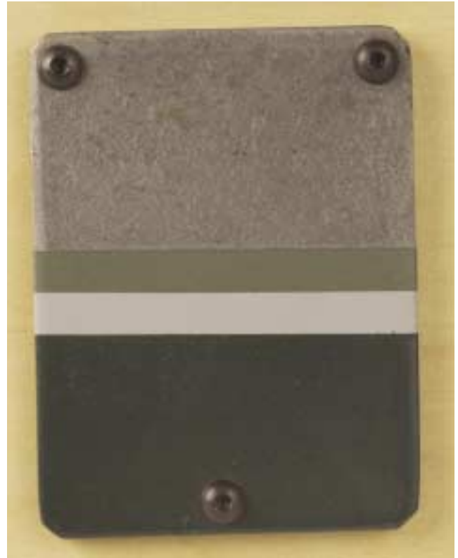
High-end primer/finish coating: polyurethane finish coat with an epoxy intermediate coat and zinc rich primer over an SSPC-6 surface preparation.
