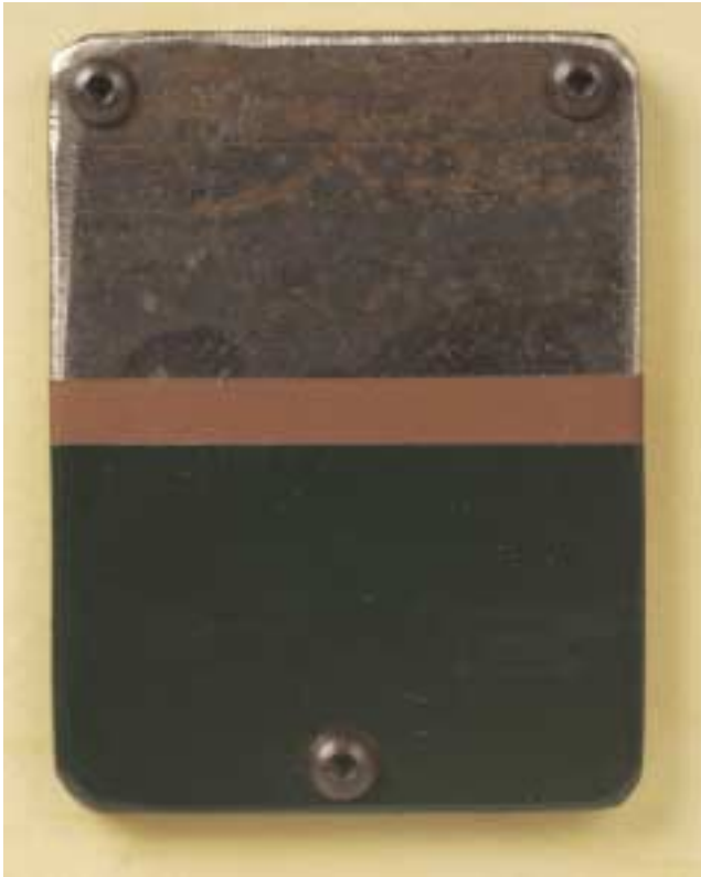
Low-end primer/finish coating: alkyd (oil-based) finish coat with a shop-coat primer over an SSPC-3 surface preparation.
