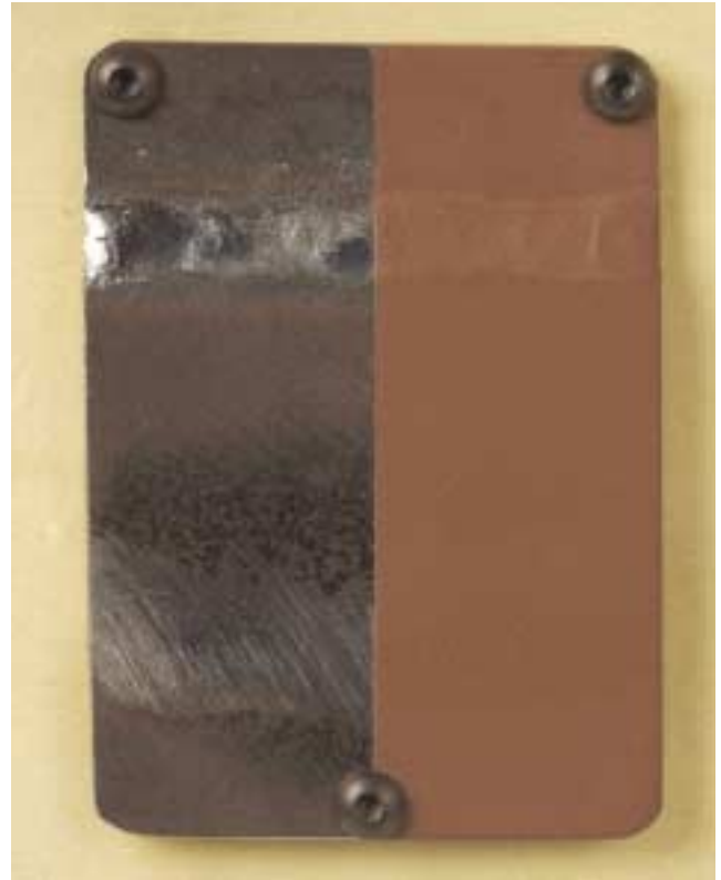
Weld show-through has been minimized.
