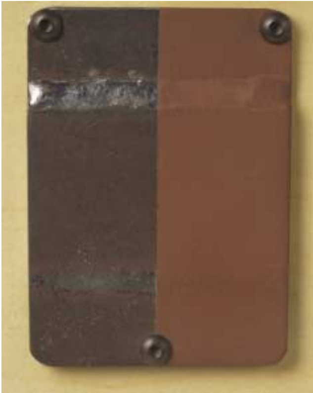
This sample shows typical weld show-through from welding the connection on the far side of the piece.
