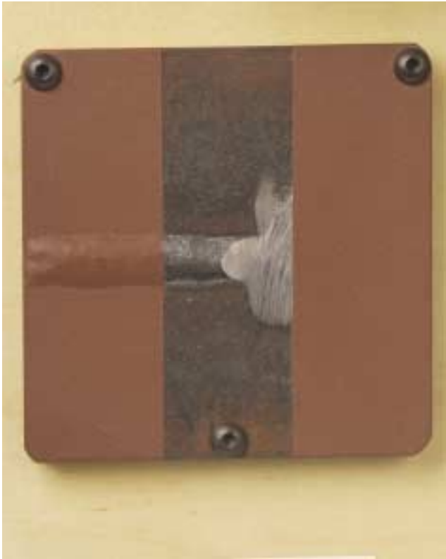
The left half of this sample shows a typical groove weld. The right half shows the same weld ground smooth.
